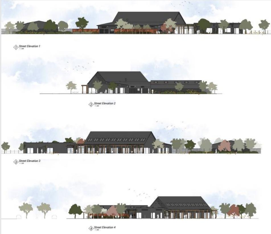
The Visitor Centre concept is based on two splayed wings with a connecting entrance foyer. The northern wing will be conceived as a barn, referencing the local vernacular while the southern wing has a flat roof supporting photovoltaics.
