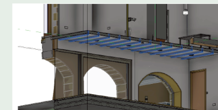
Re-point joist ends
